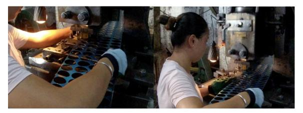
Then comes the forming process to shape the head of the spoon using the system of hammerblows. The spoon is hammered by clipping presses to repeat the desired depth shape identically.
